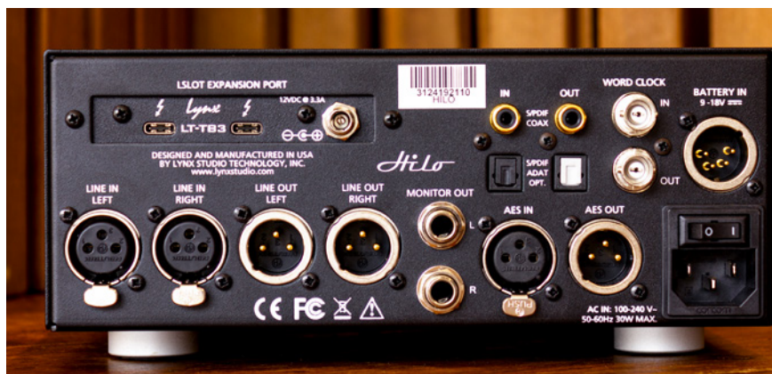
■ The expansion slot accepts USB, Thunderbolt or Dante cards, with USB being the most affordable option.
