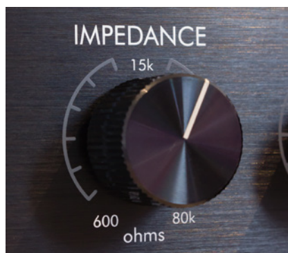
■ The Solo MPA's wide-ranging impedance control can coax different characters from some mics.
