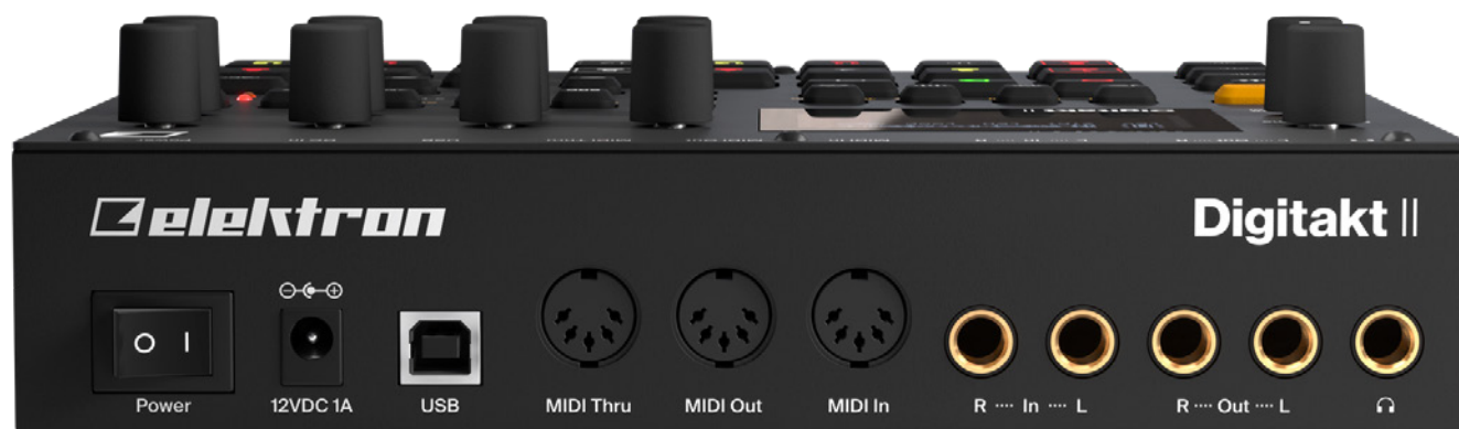
Round the back, things are identical to the Digitakt I, with MIDI in, out and thru ports and stereo audio I/O and headphone output all on quarter-inch sockets.
