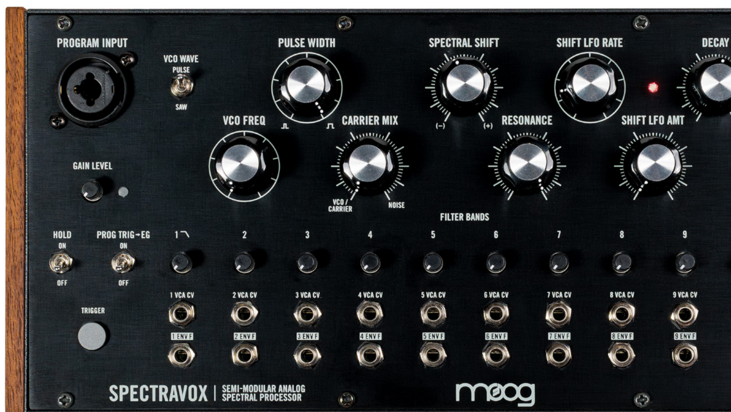
Like the other models in the range, the Spectravox's front panel is 60HP wide and can be removed from the case and fitted into a Eurorack system.
