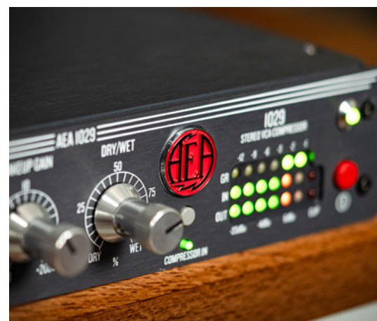
■ The dry/wet mix control makes parallel compression easy — and with the superb transient control of this compressor, it can be really effective.
