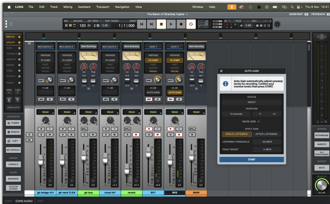
The Volt 876 is smoothly integrated into LUNA. Here, I've launched Auto-Gain on one of the inputs from a second 876 in ADAT + Host mode.
