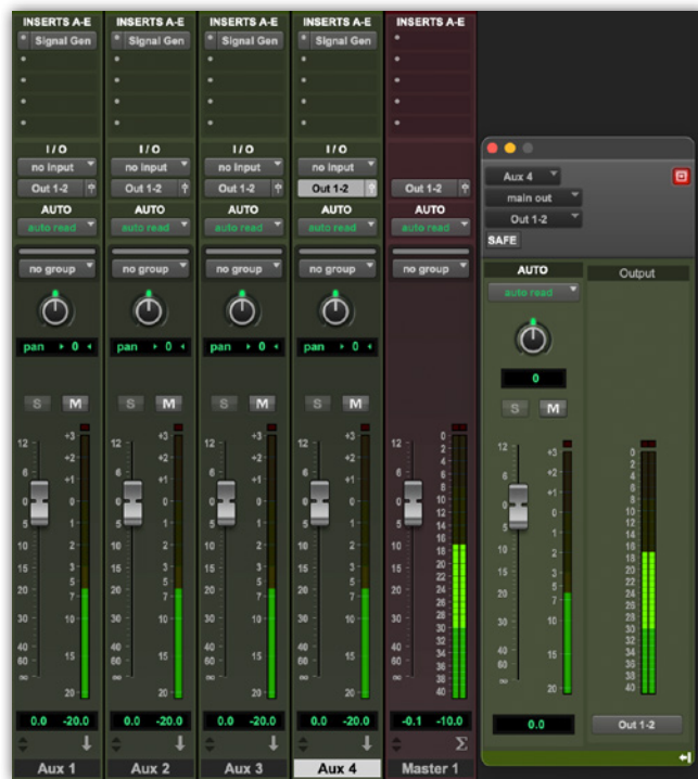
■ The expanded output window (shown here on aux 4) features the same type of metering as a Master Fader.
