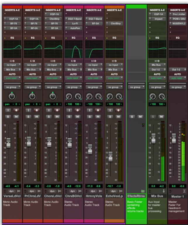
■ In this screenshot, the mix bus processing is carried out on an aux input fed by an internal bus (labelled Mix Bus), which in turn is routed to Out 1-2 and controlled by a Master Fader.
