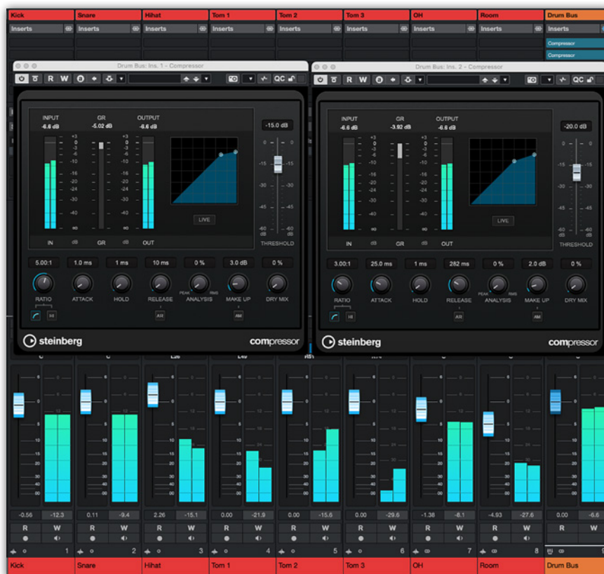
With two instances of Compressor on your drum bus, you can both tame transients and add some extra punch, without losing the natural sound of the kit.
