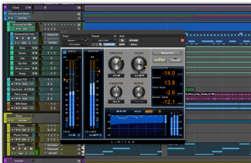
Avid's Pro Limiter has loudness and true peak metering, and is best placed on a Master Fader where the inserts are post-fader.
