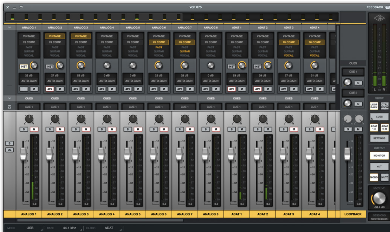
When the 876 is used as an ADAT expander, Host mode allows it to be controlled from within UA's Console, as shown in this screen capture — note that the same preamp controls appear at the top of the ADAT channels as on the first eight channels.
