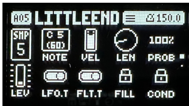
A first for Elektron sequencers: chance, fill and trigger conditions have independent slots.
