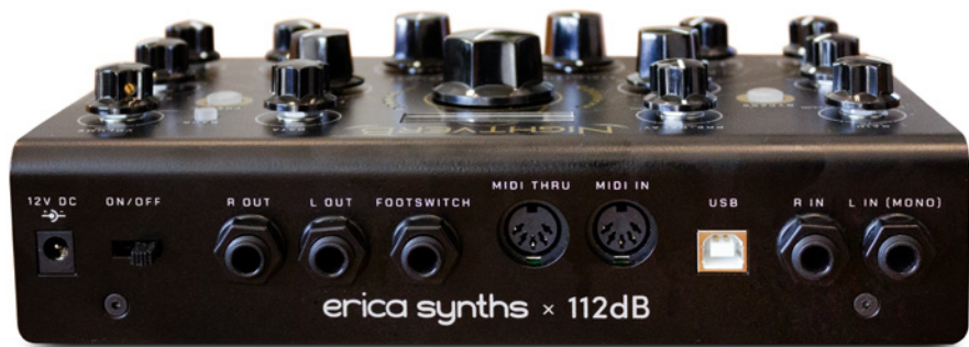
■ The MIDI thru port can be used to send MIDI CC data from the Nightverb's knobs.
