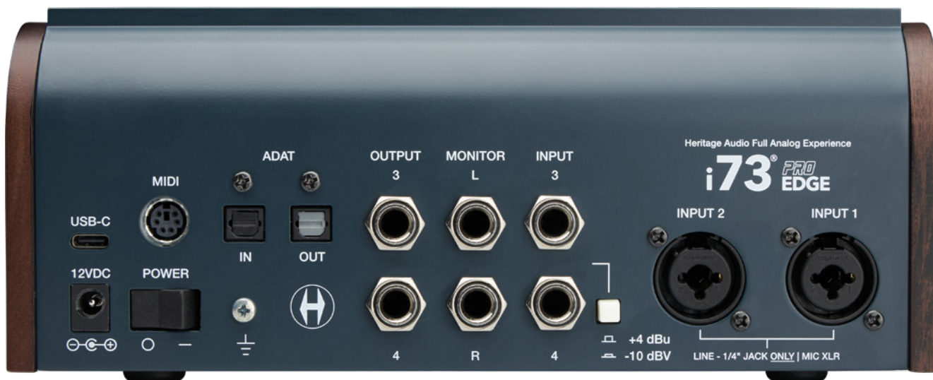
■ The flagship i73 Pro Edge features a second pair of line-level inputs and outputs as well as ADAT I/O. A special adaptor cable is needed to use the MIDI ports.
