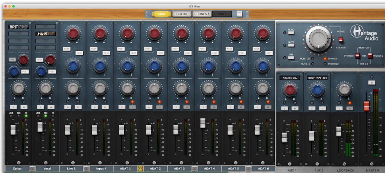
■ The i73 Mixer utility. The first two input channels have insert slots where Heritage's DSP plug-ins can be loaded, while the two auxiliary channels (right) can each host a single VST plug-in.
