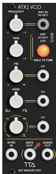
■ The ATX-1 VCO can be switched between ART, V/oct and LFO Modes.
