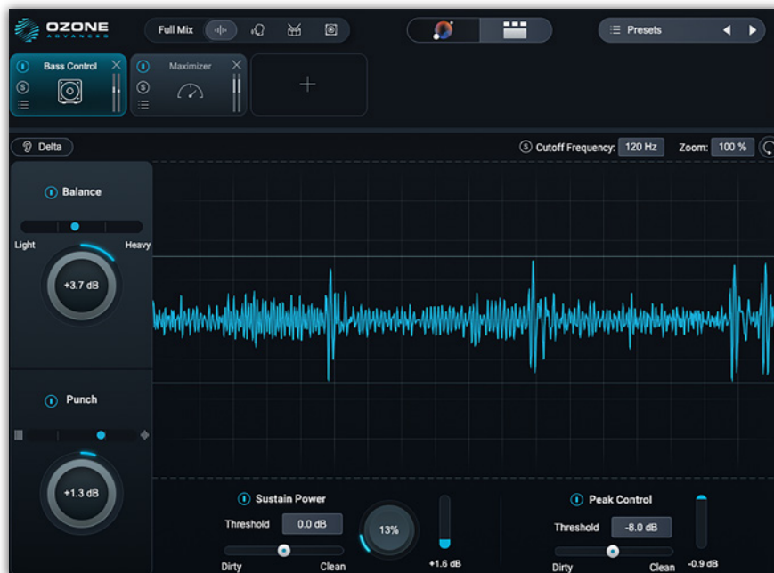
The new Bass Control module provides impressive control over the balance and dynamics of the low-frequency range while mastering.
