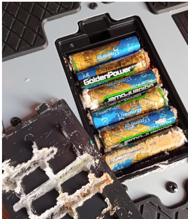
A bad case of 'the crusties' on a delay pedal that doesn't see enough use!
