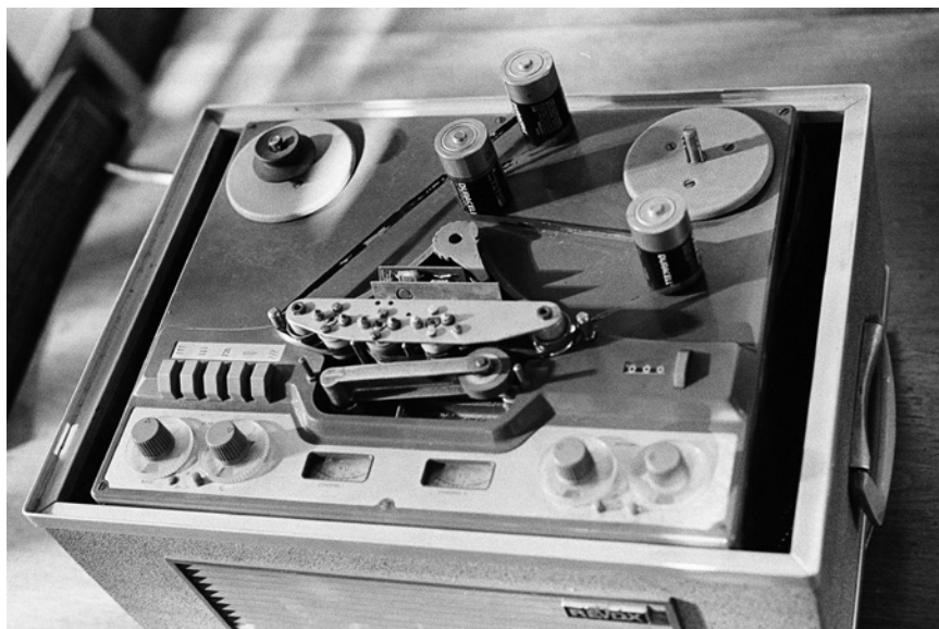
Basinski used D-cell batteries to tension the loops on his Revox G36 tape recorder.
