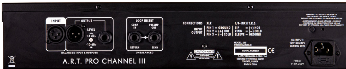
As well as the XLR mic input, there are balanced outputs on TRS jack and XLR, and there are separate TS jacks for the unbalanced insert send and return.
