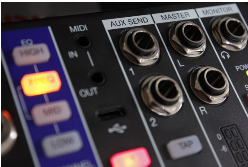
■ There are two aux sends, which can be set to operate pre- or post-fader.
